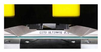
This new cutting technology, which automatically chamfers the creasing matrices on the cut edges, requires virtually no additional working on the cutting plate. European customers have unanimously confirmed that creasing matrices cut with the AC 3 Cutter could be used immediately and without any further handling.
