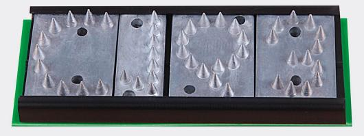
CITO Spikes are perforating tools whose distinguishing features are very easy and convenient handling. These Perfa types are characterised by extreme stability and a uniform shape, which helps to prevent outlines in the material to be cut. There is no risk of injuries due to the self-adhesion as an installation aid and extremely easy handling of the spikes when exchanging them in the rail.
