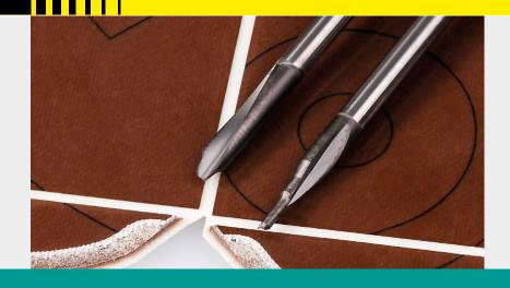
Compared with standard cutting tools, our high-speed channel milling cutters have up to 10x longer service life! With our high-speed channel milling cutters, you can achieve cutting edges in the matrices that are smooth and completely free from burrs.
